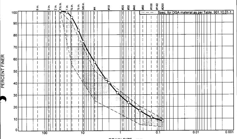
GRAIN SIZE - mm. % Fines % Gravel % Sand % +3" Clay Silt Coarse Coarse Medium Fine Fine 8.0 11.8 37.4 17.1 20.3 0.0 5.4
