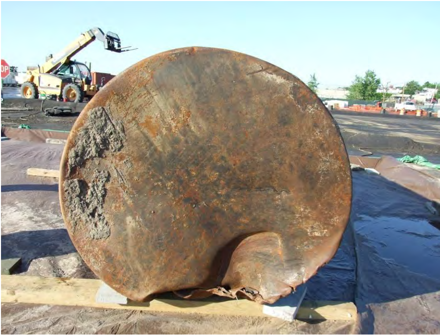
Photo 3 – View of 2,000-gallon UST removed from IRM # 1 Grid B1B. Note gash in side caused by excavator during removal.
