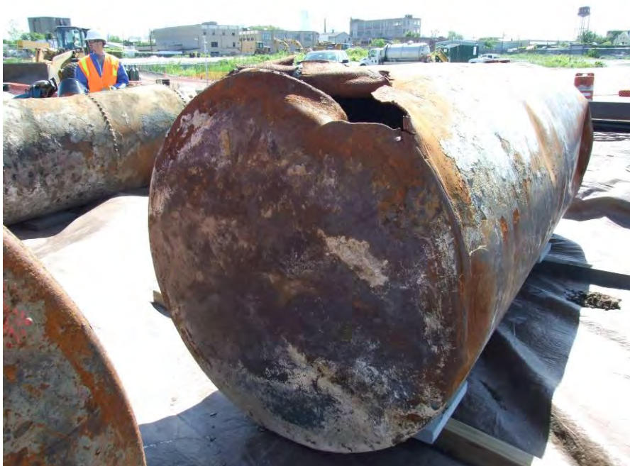
Photo 12 – View of 1,000-gallon UST recovered from IRM #1 Grids E3B / E4B. Note, large gash in side of UST caused by excavator during removal activities. Other than the gash at the seams, no corrosion holes or pitting were noted.
