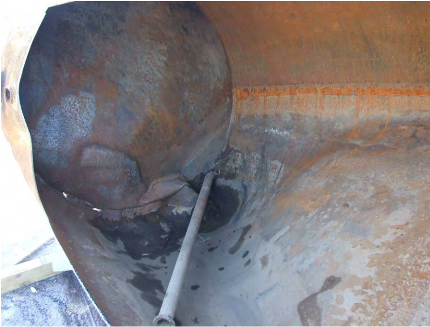
Photo 5 – View of 2,000-gallon UST interior after cleaning. Note, hole opening at seams caused by excavator during removal activities. No corrosion holes or pitting was noted.
